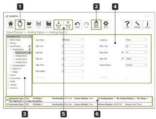
1 Single solution for all devices ConfigPilot is capable of configuring the entire ControlMaster range. Simply select the product you are creating a configuration for.
